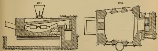
it communicates with the external air. On the crown of this arch, extending right and left, a level course of brickwork, called the cramp-course, is laid; and on this are placed iron cramps, which hold the lower ends of vertical wrought-iron standards. Upon the cramp-course a concave bed of common brickwork, grouted with lime mortar, is raised solid, sloping from the back as well
